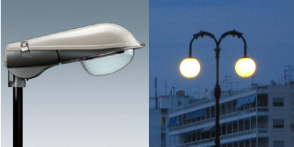
Figure 30: Luminaires with high utilization factor (left) and luminaire with very poor utilization factor due to the high upward light output (right).
