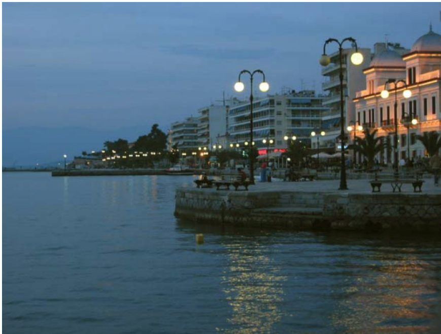
Figure 23: More than half of the light is directed to the sky or sea and is wasted
