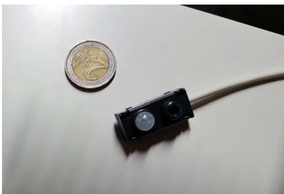
Figure 10: Helvar Active+ Sense and a coin for scale. PIR sensor is on the left and light sensor is on the right.
