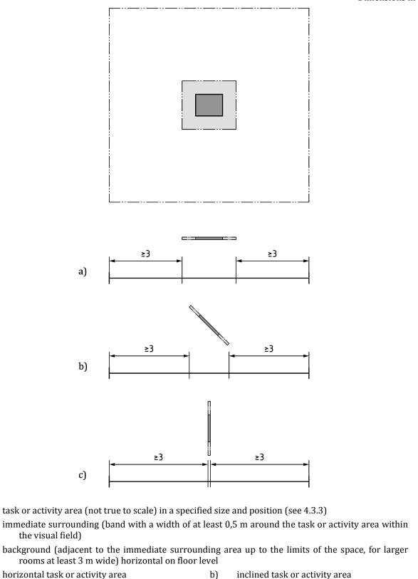
Figure 1 — Minimum dimensions of immediate surrounding and background area in relation to task and activity area (figure is not true to scale)
