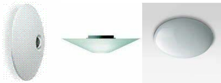
Figure 6.9: Luiminaire(left) having LOR = 83 with special finish on the PMMA screen for direct&indirect lighting Luminaire (middle) with LOR = 70 having a glass diffuser with satin finish for direct lighting versus Luminaire (right) with LOR =62 having a white colouration PMMA screen for direct lighting
