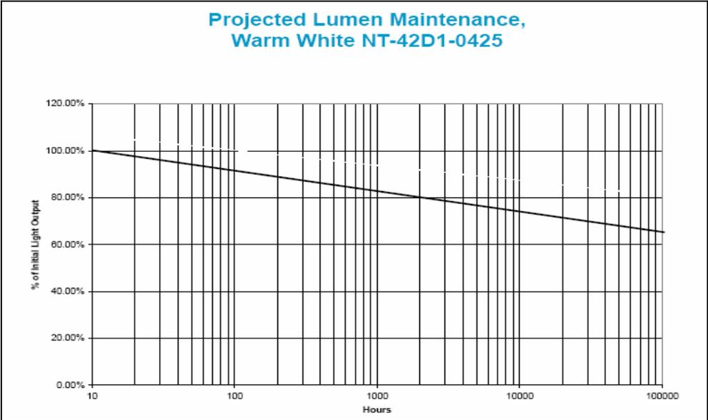
Figure 3.4: Predicted LED lumen maintenance curve for a warm white LED Source of a relatively lower quality: Atlas LED Light Engines, [www.laminalighting.com](http://www.laminalighting.com)
