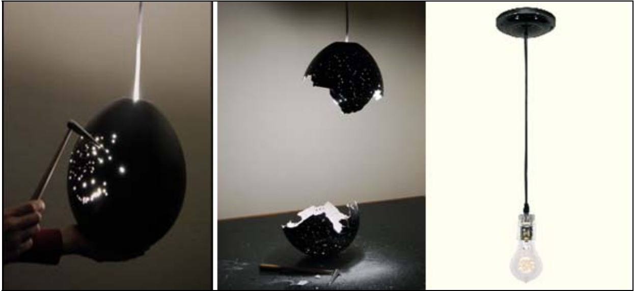
Figure 3.2 Domestic luminaire for NDLS: left with LOR < 0.1 , middle 2 LOR > 0.5 , right > 0.99
